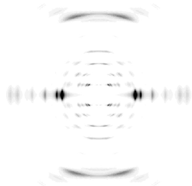
Fig. 10. Simulated X-ray fiber diffraction pattern of the refined structure of polyester 6 4 assuming a large unit cell with b parameter of 1.464 nm.
